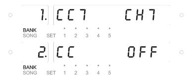
In the example shown Pedal 1 is set for control change 7 – midi channel 7. Pedal 2 is set for off.
